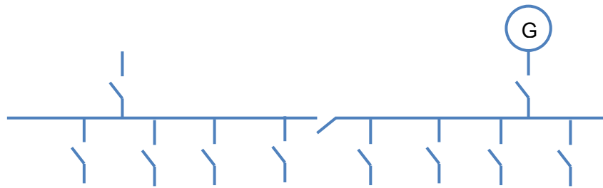
Figure 12. Scheme of a network with local generation
